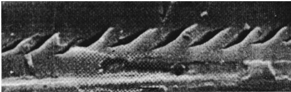
Fig. 2. Microcracks due to a shear loading (Purslow, 1981).
